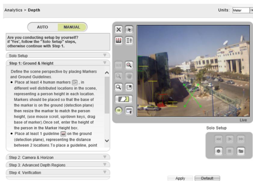
*Depth Setup Step 1: Ground & Height*
